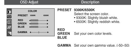
On the monitor, high gamma values display whitish images and low gamma values display high contrast images.
